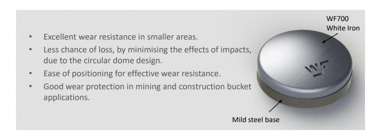
**Specifications:** Comprises of a 15/3 CrMo modified abrasion resistant white iron alloy known as WF700, metallurgically bonded to a mild steel backing plate which facilitates easy welding to the surface requiring protection. The WF700 alloy has a minimum hardness of 700 HV and a carbide network that provides its unique wear characteristics.
